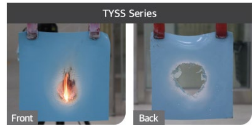
The pad remained intact, With no residual flames.
